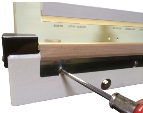
Figure 3. Loosen screws on PTFE plate.
